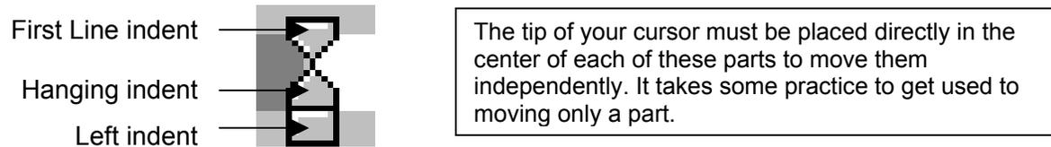
**First Line indent**—most frequently used for the first line of a paragraph in traditional formats. “Block” style format does not use first line indents.
